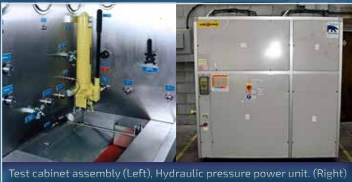
Test cabinet assembly (Left), Hydraulic pressure power unit. (Right)
