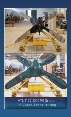
The Environmentally Protective Transport & Storage (EPTS) Aero-Propeller bags have been designed and developed for use on the Hamilton Sundstrand 54H60-91/117/77 installed onto the Lockheed Martin C-130E to H Hercules & P3 Orion Aircraft Platforms and the Dowty R391 Propellers installed onto the Lockheed Martin C-130J Hercules & Alenia C27 Spartan Aircraft platforms.
