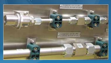
A small flow control needle valve is mounted in line with the low flow flowmeter.
