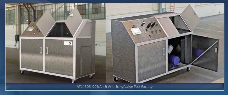
The compact, mobile, user friendly and cost effective Air Valve test facility has been designed for a modern and safe postoverhaul testing capability of air and anti-icing solenoid valves used within the Alison T56-A14/A15 Turbo-prop engines.
