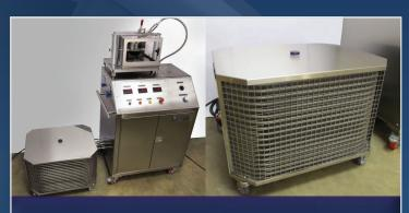
Fuel Nozzle Spray Pattern Test Facility Front View (Left) Fuel Nozzle Spray Pattern Test Facility Chiller Unit (Right)
