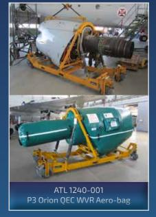
The WVR Aero-bag has been designed and developed based upon the same technology used for the ATL1175-001 C-130J WVR Aero-bag which was tested and approved by Lockheed Martin Aeronautics Inc, Marietta, Georgia. This product has consequently been identified as the preferred design for all future QECU preservation, storage and transportation standards.
